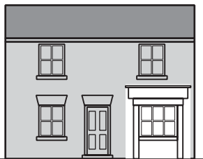
Pilasters continued down to the ground.
