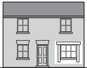
Enlarged window, with emphasised surround.
