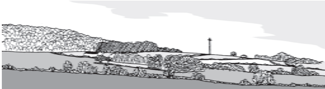
Fig. 2a Poor location for mast: skyline, on only open ridge
