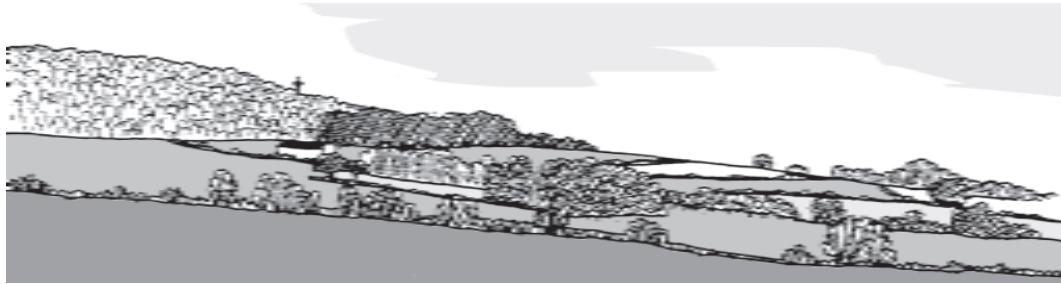
Fig. 2b Better location for mast: skyline, but most of mast concealed within woodland managed under shelterwood system for permanent standing woodland
