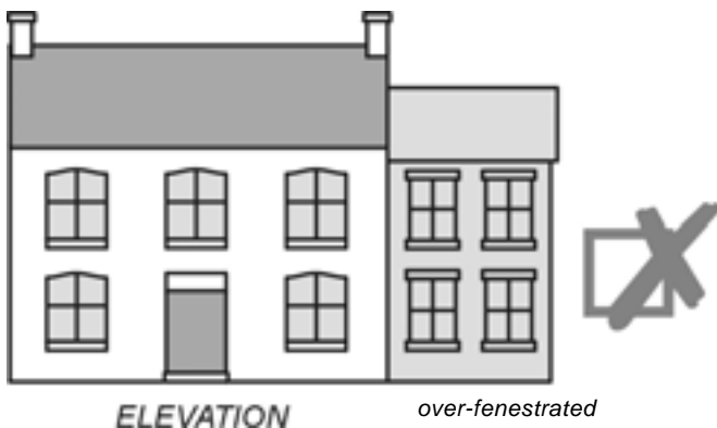
A mock-Georgian bay has replaced the original vertical sliding sash window - to the detriment of the facade.
