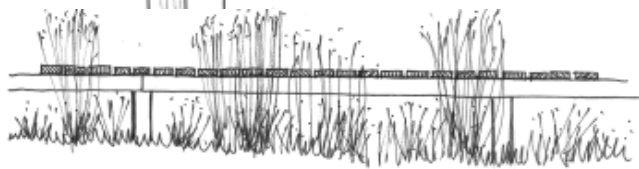
spacing of posts dependant upon strength of stringer - (usually between 1 & 2m)
